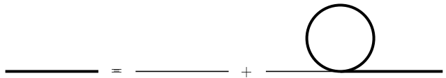
FIG. 4: Schematic representation of the self-energy contribution to scalar propagator in the self-consistent Hartree approximation. The full or ‘‘dressed’’ propagator appears as a sum of the bare propagator, and the self-energy insertion.
